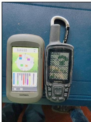
**Image 6.** Verification in the measurement of geographic coordinates from the two equipment to be used in the field. A new GPS is used as a reference.
