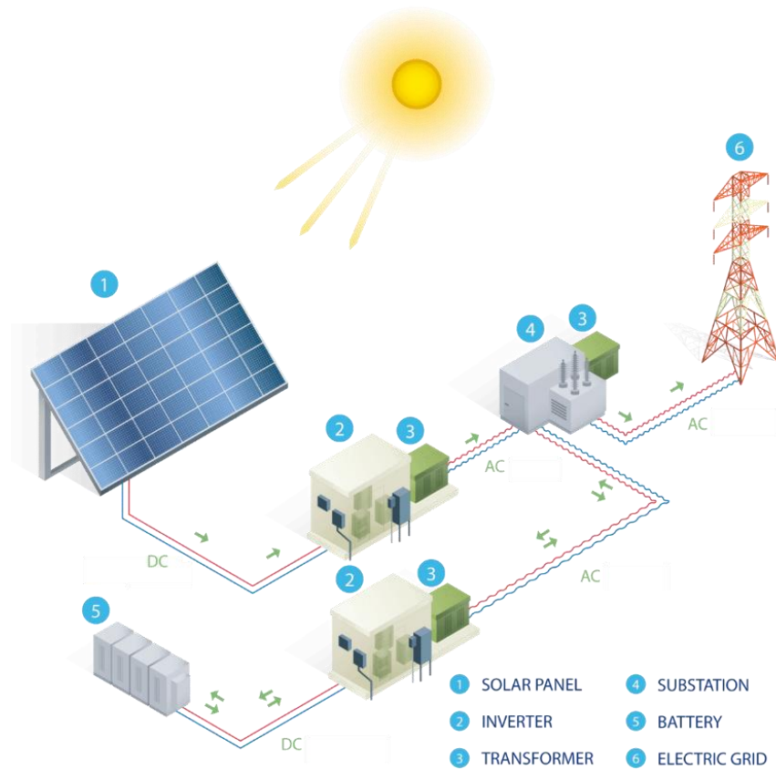
Figure 2: Basic operation diagram of a grid-connected photovoltaic installation. The Battery Energy Storage System (BESS) shown in the diagram does not apply to the project and is only schematic.
